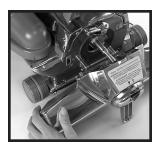
5 Place the hooks located on the rear of the nozzle over the Attaching Bar  $^{(2)}$  and push the nozzle up against the *Sentria*<sup>®</sup> system.
