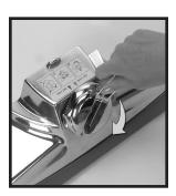
2 Release the belt tension by using the handle on the Belt Lifter to turn it all the way to the right (clockwise) until the green arrows line up.
