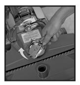
6 Push the nozzle up against the unit and turn the Accessory Lock <sup>(2)</sup> to the right (clockwise) to lock the nozzle in place. To engage the belt, use the handle on the Belt Lifter to turn it all the way to the right (clockwise) until the green arrows line up. Then lower the Headlight Hood <sup>(2)</sup>. ►
