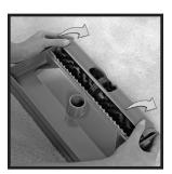
7 To clean the brush, push the thumb pads located at each end of the plastic shield and rotate the shield up and away from the brush.
