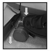
9 Press the Toe-Touch Control Upper Pedal (8) to lower the brush one notch at a time. Lower the brush as far as the Toe-Touch Control will allow.
