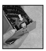
3 Align the metal ends of the brush with the slots on the tray and push the brush in until it snaps into place. The brush will only fit the tray the correct way.
