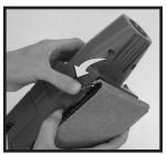
Tightly wrap the paper around the bottom of the Turbo Accessory and tuck the end into the rear clamp. Lock the rear clamp.  $\blacktriangleright$
