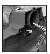
5 While sliding the Carpet Shampoo System Nozzle/Tray Assembly toward the *Sentria*<sup>®</sup> system and over the Motor Shaft <sup>(2)</sup>, connect the hooks on the bottom rear of the nozzle to the Attaching Bar <sup>(2)</sup>. ►
