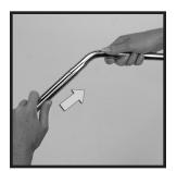
5 If desired, prepare the long waxer roller handle for storage by depressing the spring-loaded pin on the lower portion of the handle while pushing the upper portion toward the hooked end.
