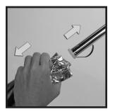
5 Grasp both the packing bag and roller firmly and pull them off the long roller waxer handle. To do this, push the roller away from the handle grip toward the bar to compress the retaining spring. This will allow you to slide the roller over the end cap. Seal bag tightly to prevent premature drying. Store in the provided packing tube and put in a safe place away from children and pets until next use. ►
