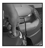
2 Turn the Suds Control Valve all the way to the right (clockwise) to the ON position. Turn the *Sentria* system ON and engage Tech Drive<sup>®</sup> power assist (see page 7 for details). Suds flow will begin immediately.
