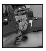
Belt Lifter to the left (counter-clockwise) until the red arrows line up. ►
