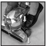
3 Lower the Carpet Fluffer Nozzle one notch at a time by pushing the Toe-Touch Control Upper Pedal ⑧. The instant the brush contacts the carpet, stop lowering the brush. ►
